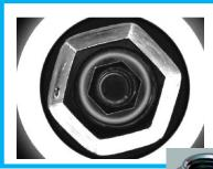
↑ Total outer inspection with just one camera for nuts
