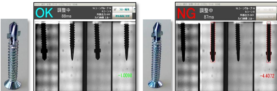
M4X35mm Phillips recess OK and tip shape NG samples
