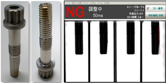
M8X35mm Engine bolt thread damage sample
