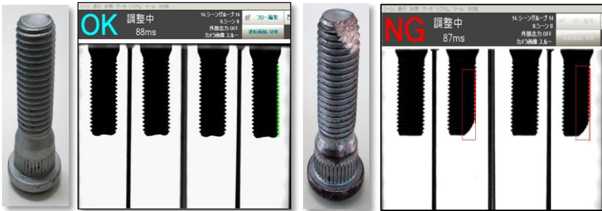
M14X40mm hub bolt OK and tip damage NG samples
